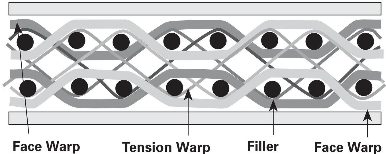
***PolyVynlok utilizes a Solid Woven Carcass with PVC and Spun Polyester Binder Warp (Face Warp) and PVC and Filament Polyester Tension Warp. The filament offers High Tenacity-Low Stretch and both yarns have Moisture-Acid-Oil Resistant properties.***
