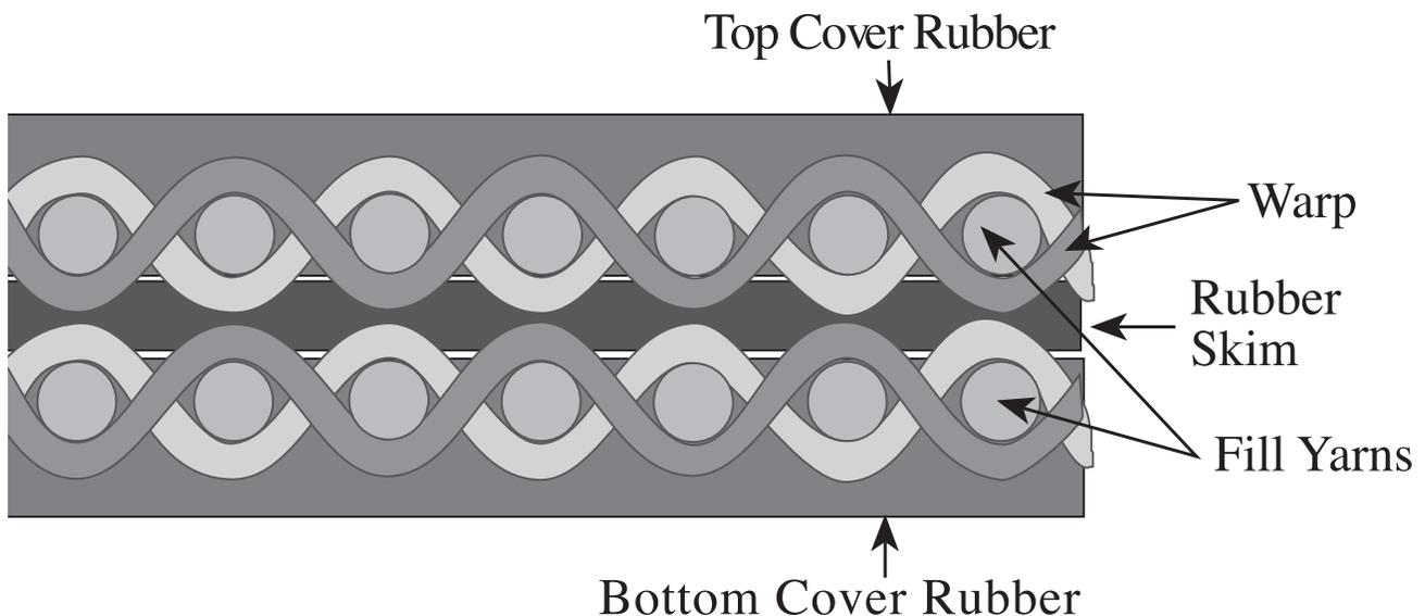
as many layers as is required to provide the necessary belt strength...usually bound together with rubber.
